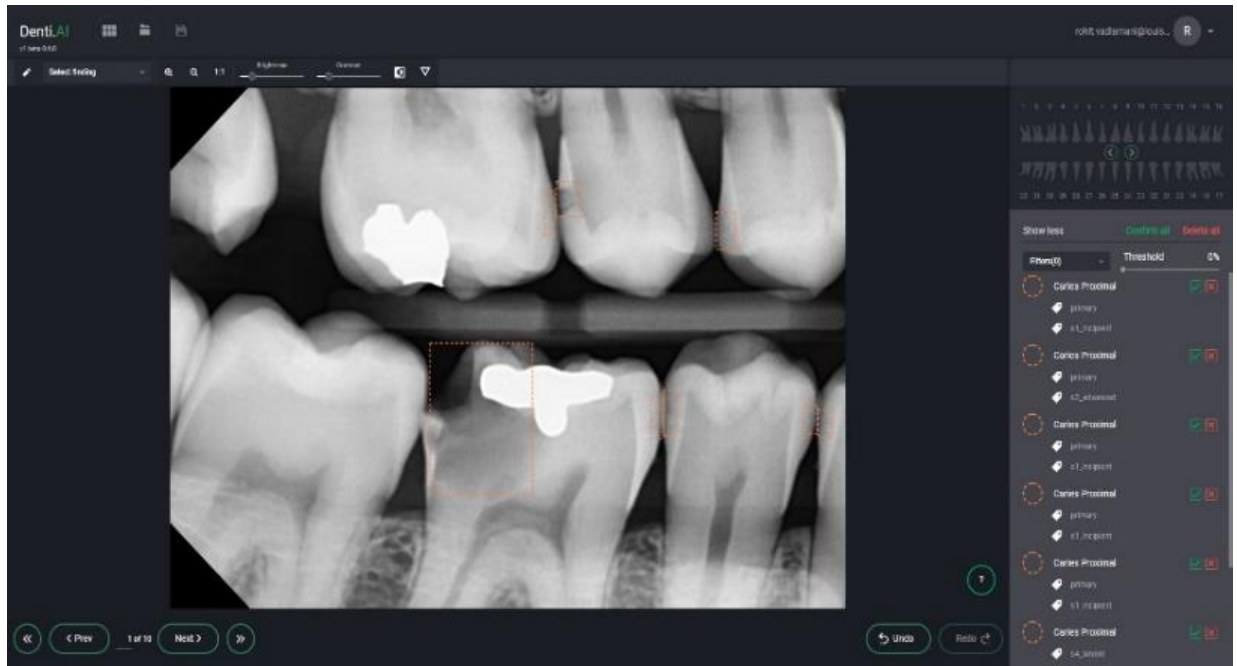
Fig 1. Denti.AI Software Interface. Screenshot of Denti.AI interface shows annotation of the presence and location of proximal lesions (red rectangles) and tagging depth in right column (by experts only).
